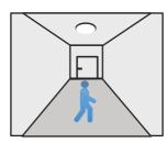
When the motion is detected with sufficient daylight (>300LUX), the light remains OFF.
